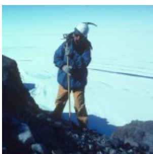
Barry McKelvey using a Jacob's Staff to measure a section through Pagodroma Group.
