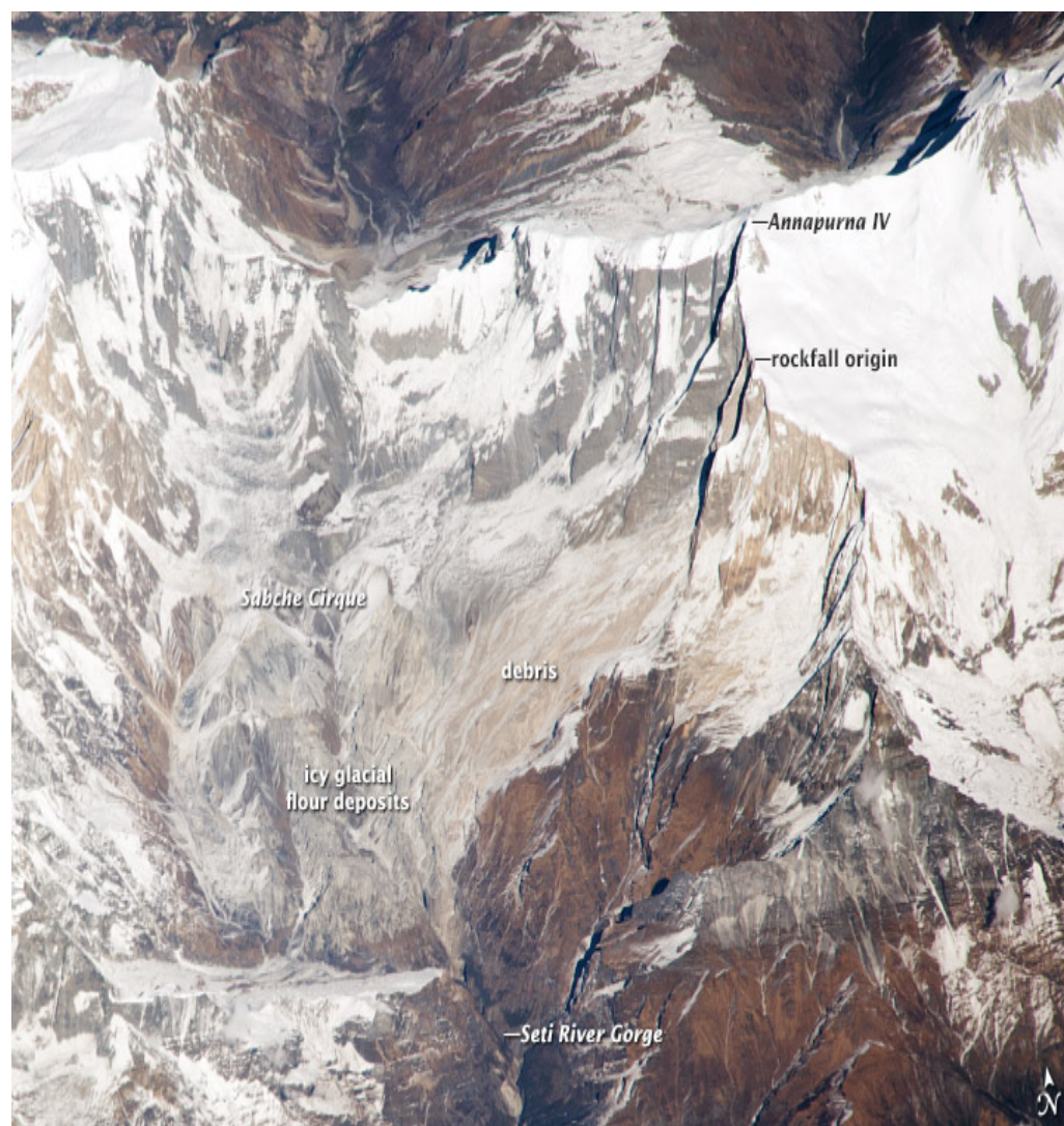
Figure 3: Aerial image to illustrate the origins of the rockfall in the Sabche Cirque. Photo credit: Public domain, via Wikimedia Commons .
